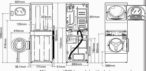
\*Non-coin (OPL) model with drain pump shown
